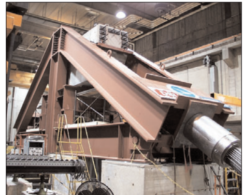
Full scale test of the 119-strand cradle in the CTL testing lab. The cradle stay system was pre-purchased from DSI.
