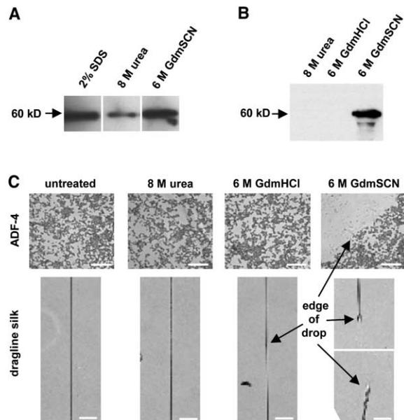
Figure 3. Chemical Stability of ADF-4 Aggregates, Filaments, and Dragline Silk Threads
